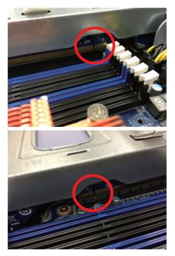
• If the GPGPU card supports 225W, connect 2 x 4 power cable.
