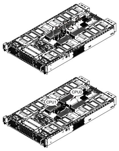
CPU0 and CPU1 use the different CPU heat sinks. Please see the following table for installing the correct CPU heat sink.
