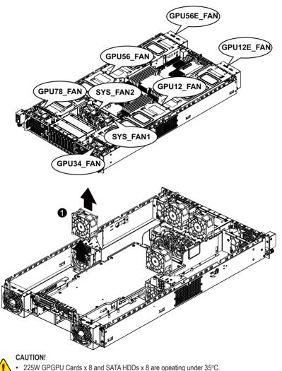
• 300W GPGPU Cards x 8 and SATA HDDs x 8 are opeating under 30°C.
