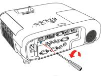
Insert the wireless LAN module into the USB-A port.
