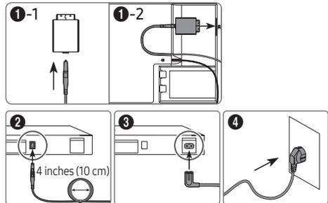
Refer to the picture and connect the MICRO LED and One Connect Box with the One Connect cable provided as a component.
