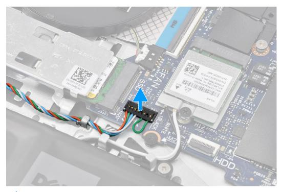
**NOTE:** For models shipped with a speaker cable featuring an eight-pin connector, to disconnect the speaker cable from the system board, pry up the bottom side of the cable connector's head first and then pull it away from the connector.
