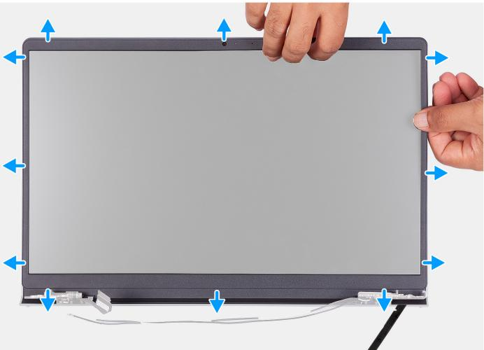
1. Using a plastic scribe, pry open the display bezel from the outer edge of openings at the bottom side of the display assembly, near the display hinges.
