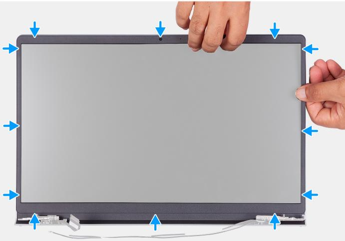
Align the display bezel with the display back-cover and antenna assembly, and then gently snap the display bezel into place.
