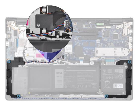
**3.** Connect the speaker cable to the system board.
