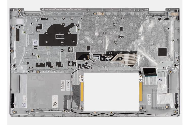
Place the palm-rest and keyboard assembly on a flat and clean surface and perform the post-requisites to install the palm-rest and keyboard assembly.
