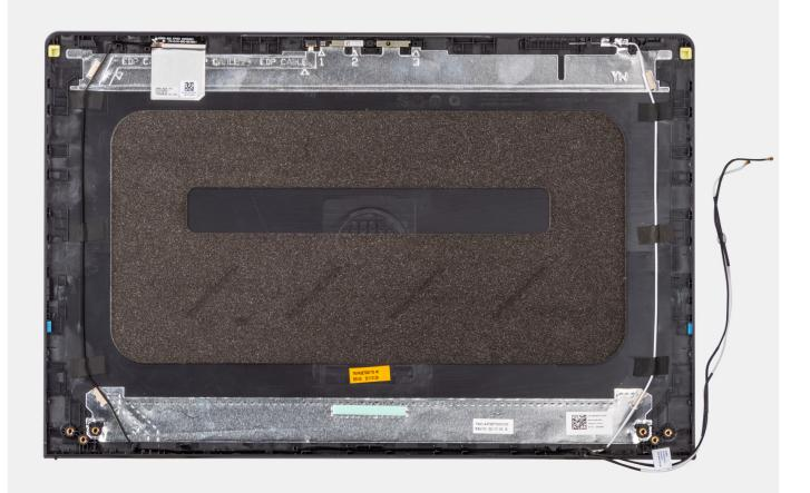
After performing the pre-requisites, you are left with the display cover and antenna assembly.
