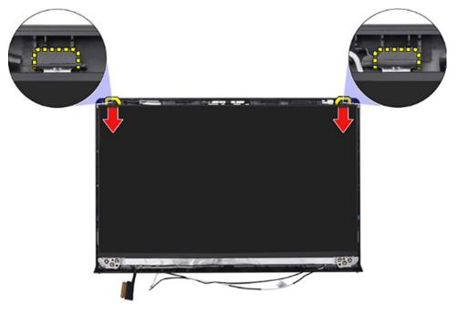
5. Gently flip the display panel assembly forward, peel back the Mylar tape securing the display cable on the rear of the display panel.
