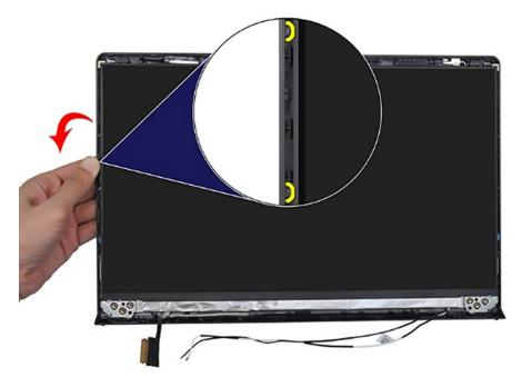
4. Lift the bottom side of the display panel and slide it downward to release the display brackets from the slots at the top side of the display cover.
