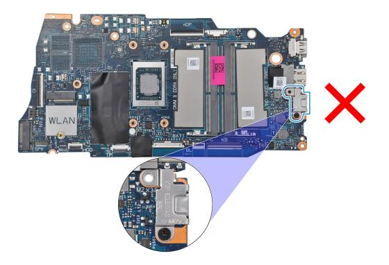
7. Carefully lift the system board away from the chassis.
