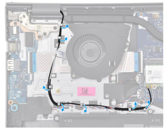
5. Route the speaker cable through the routing guides on the palm-rest and keyboard assembly.
