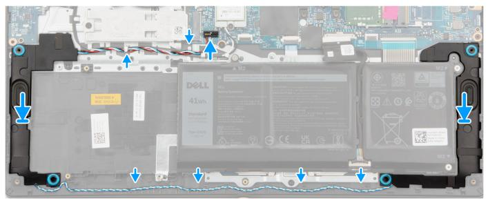
1. Using the alignment posts, place the speakers on the palm-rest and keyboard assembly.
