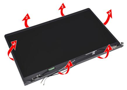
5. Lift and remove the display bezel from the display assembly.
