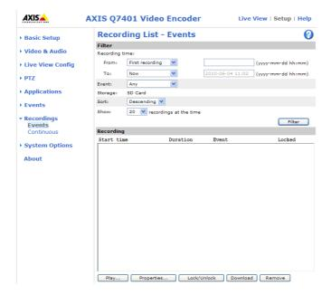
The AXIS Q7401 Video Encoder can be set to record continuously or as result of a triggered or scheduled event. See Continuous Recording, on page 34 and Event Types, on page 28 for more information. The Recording List window contains a list of recordings made to the local storage. It shows each recording's start time, length, the event type used to start the recording, and if the recording is locked so that it can neither be deleted nor recorded over.
